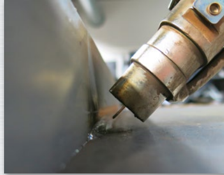
Determination of stick-out for optimal results.
