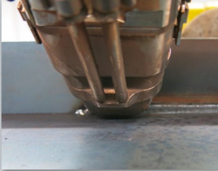
Exact positioning of the WH Tandem W 800 torch.
